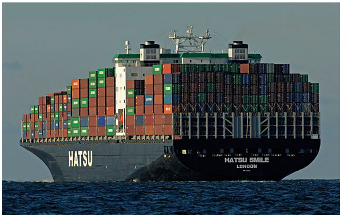
A relatively new type of vessel is the 'open top' or hatchless container ship. The advantage of the open top is that it speeds up loading and unloading times, since it is unnecessary to stop and remove the water-tight hatches
