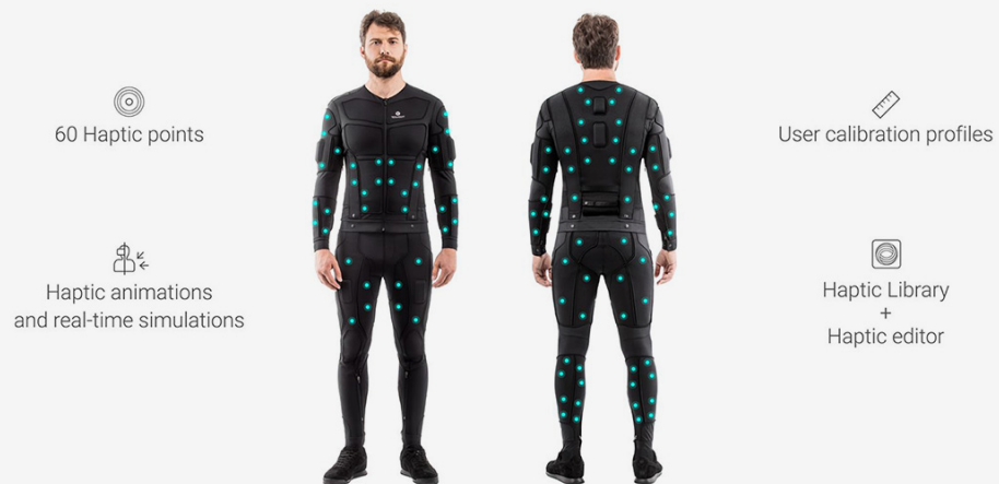
Diagram of the haptic feedback system for an early iteration of the TESLASUIT
