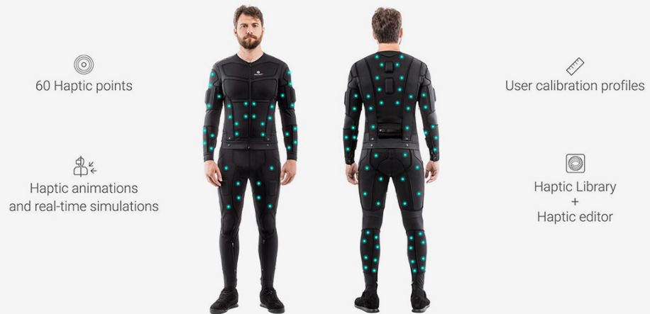
Diagram of the haptic feedback system for an early iteration of the TESLASUIT
