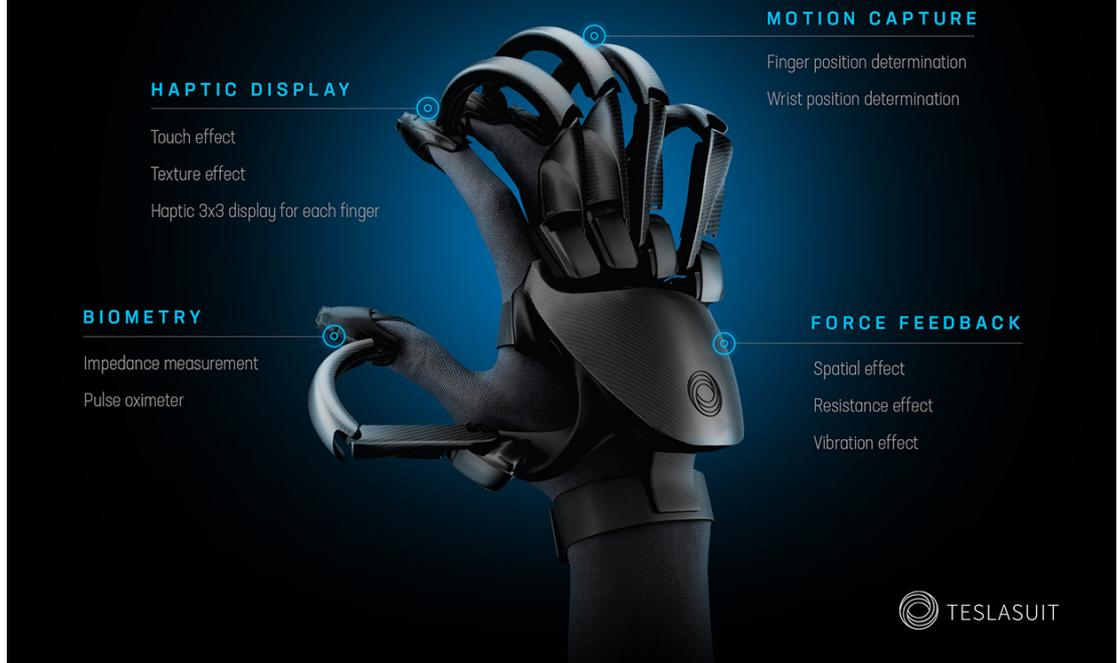
TESLASUIT Glove, an exoskeleton force feedback glove used in conjunction with the TESLASUIT
